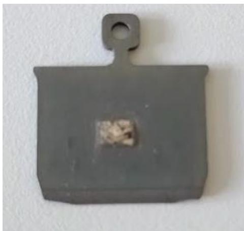
Figure 21 Omicron flag style holder compatible with the PHELIX and URANOS systems.  $\text{Bi}_2\text{Te}_3$  single crystal is placed in the middle of the holder and attached by the UHV glue.
