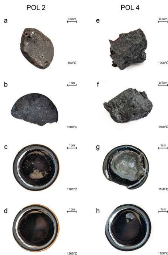
Fig. 5 Macroscopic photos of slags after the high-temperature experiments
