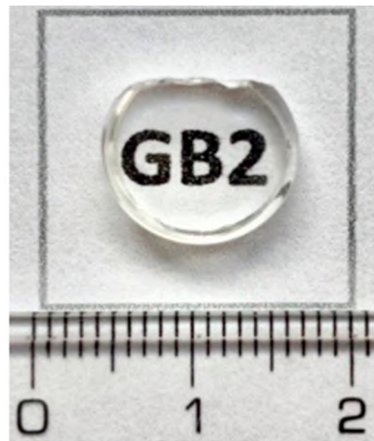
Figure 2. Photographs of the obtained glass sample: 30\text{GeO}_2\text{-}30\text{B}_2\text{O}_3\text{-}30\text{BaO}\text{-}10\text{Ga}_2\text{O}_3 (GB2).
