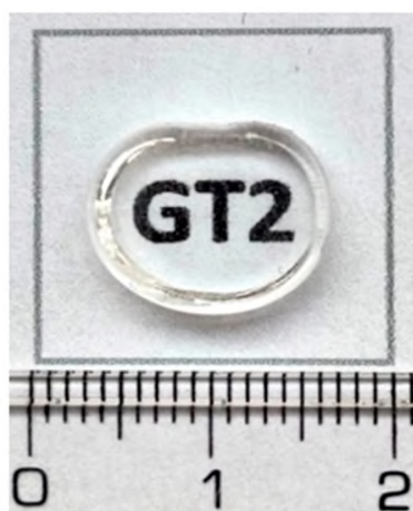
Figure 1. Photographs of the obtained glass sample: 30GeO 2 -30TiO 2 -30BaO-10Ga 2 O 3 (GT2).
